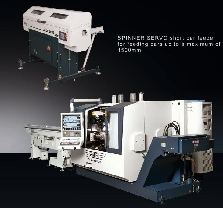
SPINNER SERVO bar loading magazine for feeding bars up to a maximum length of 3,2 metres
